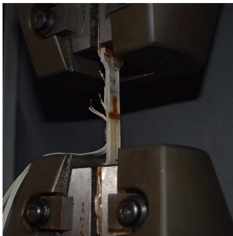
Figure 5. The positioning of the test specimen between the machine’s wedge grips
