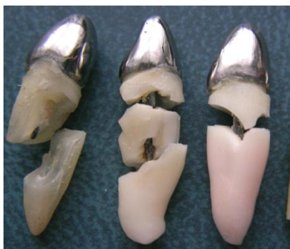
Fig. 4. Fractures in the group C (from left to right): vertical, complex and cervical fracture
