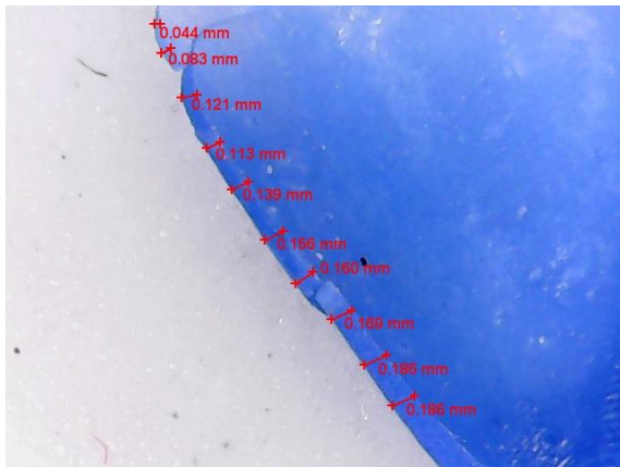
Figure 5. Measurements of the silicone thickness.
