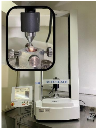
Figure 3. Universal testing machine and a specimen subjected to a compressive load
