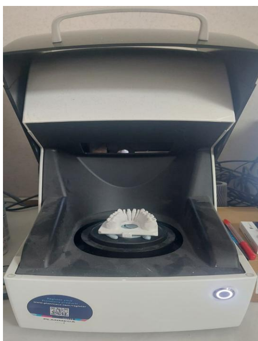
Figure 1. Scanning of the reference model using Planscan Lab (Planmeca)
