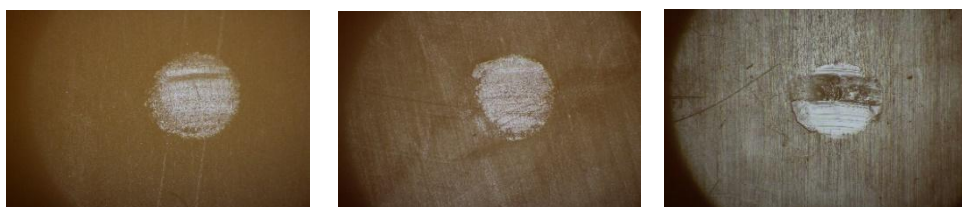
Figure 1. Optical microscope images of wear scars on resin samples with zirconia ball for half an hour in a dry environment. a)PU, b) FFC) FA
