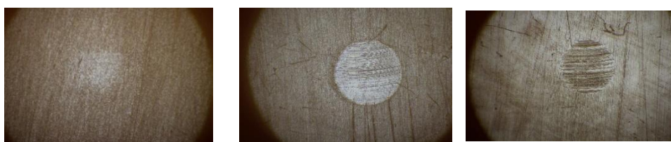
Figure 2. Optical microscope images of wear scars on resin samples with stainless steel ball for half an hour in a dry environment. a)PU, b) FFC) FA
