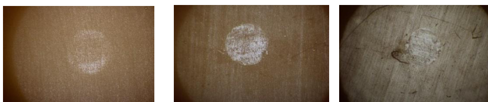
Figure 3. Optical microscope images of wear scars on resin samples with zirconia for half an hour in a wet environment)PU, b) FFC) FA
