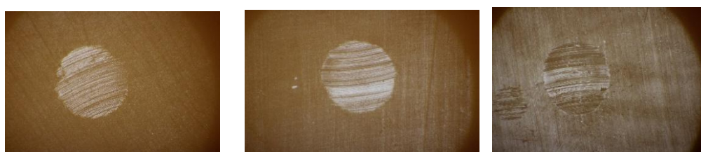
Figure 4. Optical microscope images of wear scars on resin samples with stainless steel ball for half an hour in a wet environment. a)PU, b) FFC) FA
