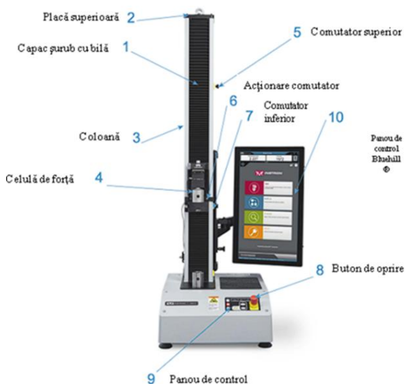
Figure 2. Tensile strength measuring device Instron 34SC-5.
