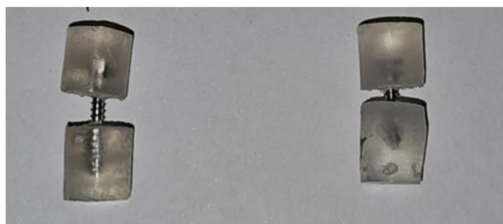
Figure 3. Samples embedded in acrylic mass for tensile testing.
