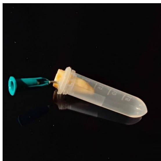
Figure 2. The cap with the tooth and attached needle
