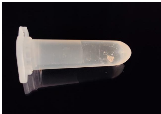
Figure 5. The debris inside the Eppendorf tube after drying in the incubator
