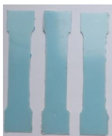
Fig. 4. Samples cut and processed from the initial circular shape (with protective foil) A total of 11 samples were stressed until failure: 4 samples made from 0.8 mm thick
