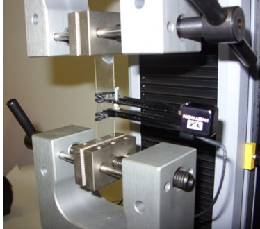
Fig. 7. Testing the samples, on the Instron type machine with the extensometer mounted
