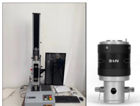
Fig. 1. The mechanical system (testing machine) used for axial tensile testing is INSTRON - 34SC-5.
