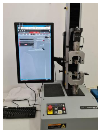
Fig.1. The system used for elasticity tests
