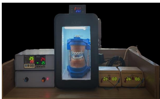
Figure 1. Scientific orthodontic simulator with temperature control and thermo controlled chamber OSIM No: A 2024 00105
