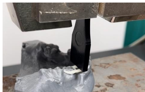
Figure 2. Compression load testing using the Zwick/Roell Z 005 machine.
