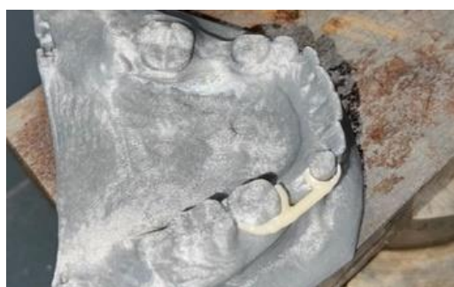
Figure 3. Fractured space maintainer after compression load testing.
