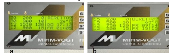
Figure 3. (a) The standard recommended sintering parameters but the heating was fast and the cooling was slow; (b) Sintering with fast heating, 12 minutes maximum temperature of 750°C followed by a slow cooling.
