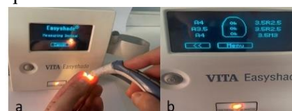
Figure 4. Colorimetric measurements of the samples of group 2 with Vita Easy Shade.
