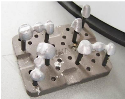
Fig.1. The metal infrastructures sandblasted, and prepared for oxidation.
