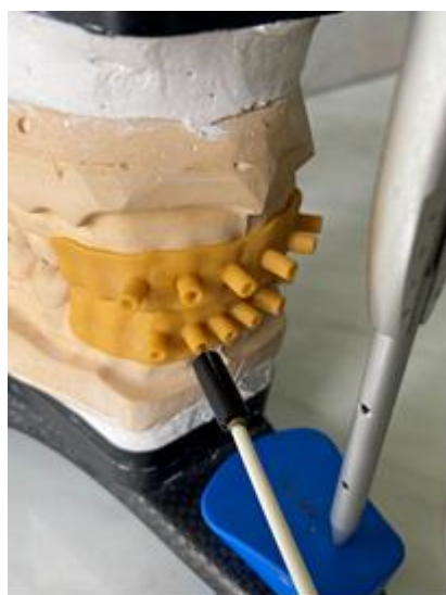
Figure 4. The probe holder with the 1mm diameter laser Doppler optical probe
