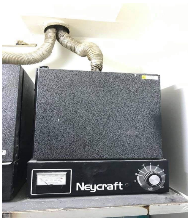
Fig. 11 – Preheating the pattern
