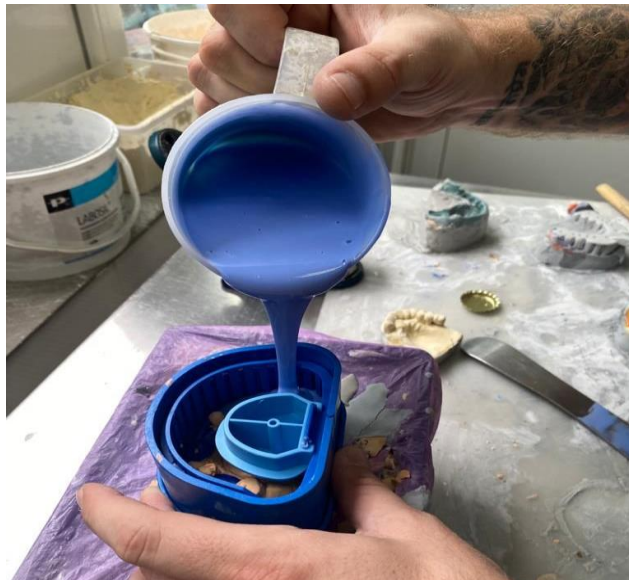
Fig. 5 – Pouring silicone into the shaper
