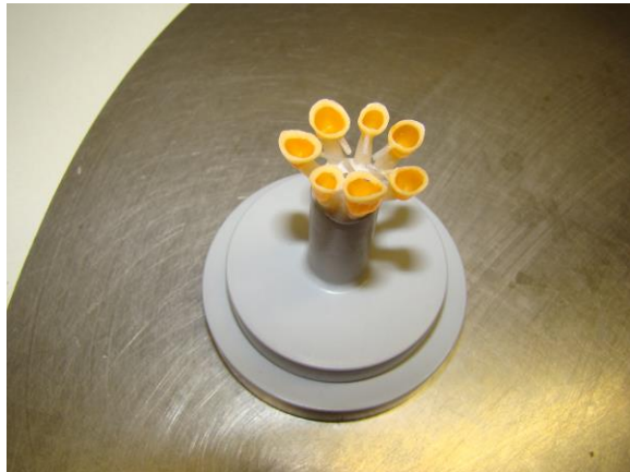
Fig.3 The wax pattern fixed in the injection device
